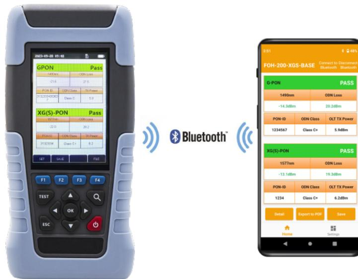
With the upgrade of GPON networks to XG(S)-PON, we have launched the new FOH-200XGS-BASE to apply for the installation and maintenance testing of the upgraded Combo PON network. By connecting FOH-200XGS-BASE to the PON network, we can quickly and accurately extract OLT information including OLT PON-ID, ODN class, Tx power, power level and ODN link loss pass/fail per ITU-T.
